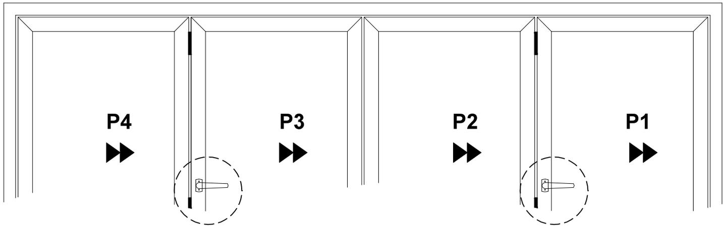
1. Starting from main swing panel, OPERATE lever handle then outward open MAIN SWING PANEL inline with adjacent center panel, allowing it to clip in to stop.
