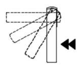
To Open bi-fold, pull handle up 90°and release then push out.
