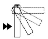
To Open bi-fold, pull handle up 90°and release then push out.
